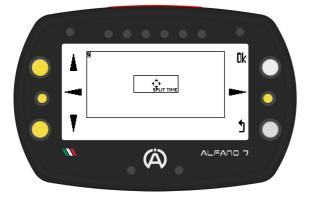
To **add** a **widget clicking** "**Ok**" (when the corresponding icon is selected) a **list will open** for **selecting** the **desired block**
