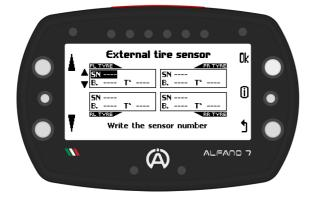
If you do not want to associate a sensor for one or more wheels, keep the serial number on "----" and press the "ok" button to confirm and move on to the next wheel
