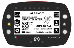
In this mode, due to the different versions of tracks in memory, the **device** will **automatically preselect possible nearby tracks**
