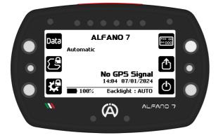
To unlock, press and hold the lower left or centre left button for 3 seconds
