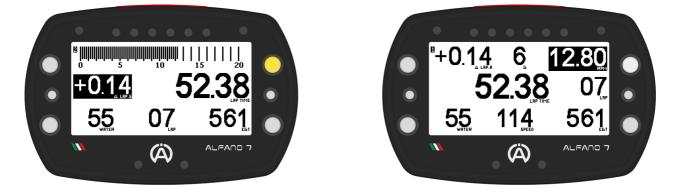
When the device enters race mode, if you have not manually chosen the desired screen in the race screen management menu, the screen used in the previous session will be shown
