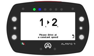
Enter the requested gear and continue learning until the last gear is reached (value entered in the previous screen under the "number of gears" item)
