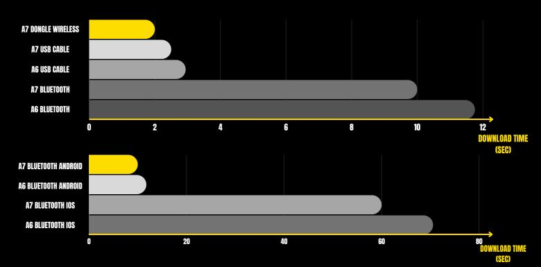
BENCHMARKS WERE CALCULATED ON IDENTICAL CONFIGURATIONS OF ALFANO 7 AND ALFANO 6, WITH CONNECTED SENSORS SET AT 10 HZ, EXCEPT For the GPS which was set at 25 Hz in Alfano 7 and 10 Hz in Alfano 6. Download times were calculated on an 8-laps session, with Each lap taking 50 seconds
