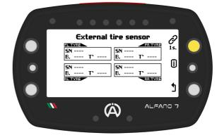
Using the lower and upper left buttons, set the serial number of the sensor you want to associate with the wheel:
