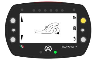
The lower right LED will turn green to indicate that the line is far enough from the existing lines on the track
