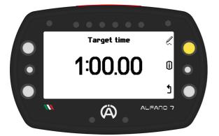
Set the desired time using the upper and lower left buttons.
