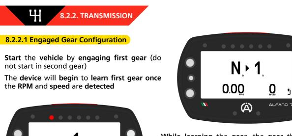
While learning the gear, the gear that the device is configuring is indicated in the center of the screen
