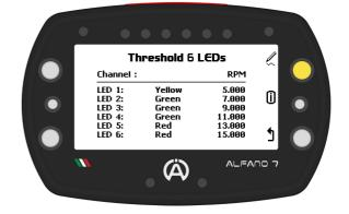
Use the upper and lower left buttons to scroll through the channels. Press the 'ok' button to modify the thresholds and LED color of the selected channel
