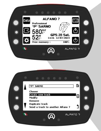
**Confirming** the "**Create new track**" item with the "ok" button will **open** the **configuration menu** for **creating** the **new circuit** if the instrument is receiving the GPS signal
