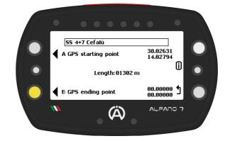
The finish line coordinates will be displayed at the bottom left. You can update the coordinates of point (B) by pressing the corresponding button again (this will update the distance traveled between points A and B)
