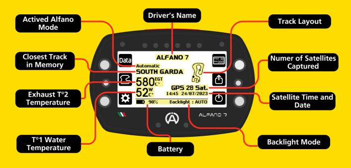
The device's available memory is displayed at the bottom of the screen, alternating with the battery charge and backlight mode
