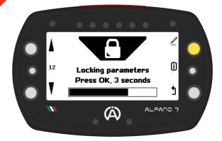
Access to the all settings menu (icon on the bottom left) and access to the Alfano mode selection menu (icon on the centre left) is not possible until the lock is removed
