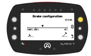
When you confirm that you want to calibrate the sensor, the cursor will move to the 80b position
