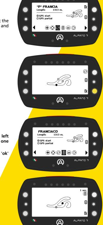
To delete the finish line it will be necessary to change the finish line with another line and then it will be possible to delete the old finish line
