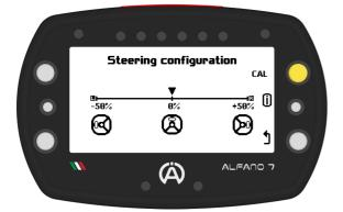
Once the position corresponding to the straight steering wheel has been recorded, the cursor will move to the +50% value corresponding to the steering wheel turned all the way to the right
