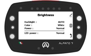
The **9 LEDs** (6 LED system, two alarm LEDs and status LEDs) can also be **adjusted** to **three levels** of **light intensity**: **low**, **normal** and **high**
