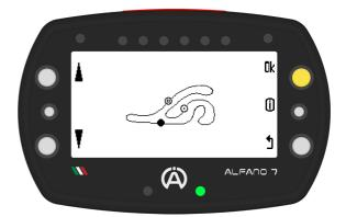
If the device does not allow you to add other lines, you have entered the maximum number of sectors for this circuit or the maximum number of sectors supported by Alfano 7, which is 9
