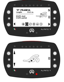
The LED indicator displays a green light if the modified line is at a sufficient distance from the existing lines on the layout, and a red light if it is too close to another line; in this case, it is not possible to exit the modification until the line is in a valid position
