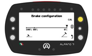
When the position corresponding to 0% is confirmed, the calibration is completed and the real-time status of the brake pedal is displayed again
